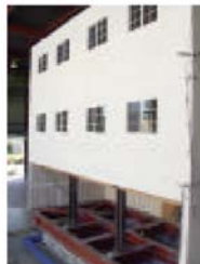
Full-scale shake table testing of a two-story house (left, UC San Diego) and three-story apartment building (center, UC Berkeley). A new engineering analysis method and software package were produced (right).
