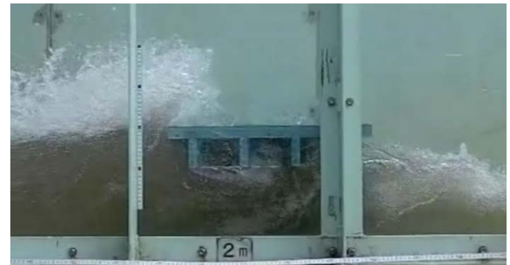
Flume test for bridge model to study response of bearing supports
