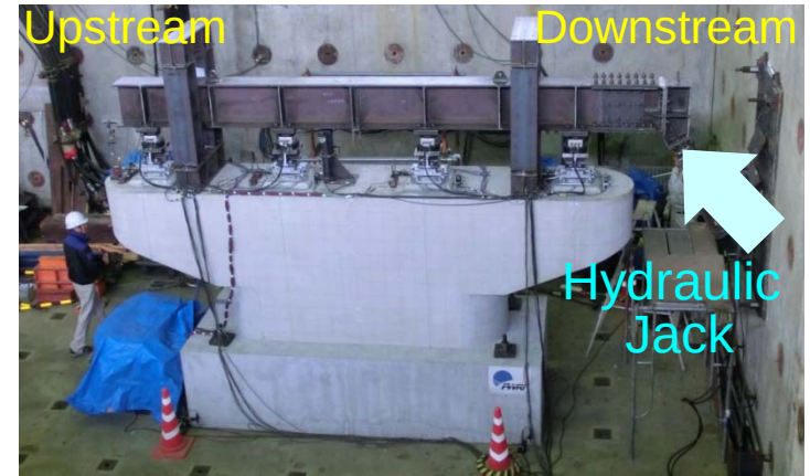
Static loading test to examine resistant capacity of bearing supports
