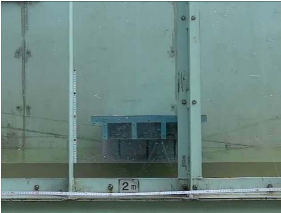
Flow pattern for 4-main girder bridge
