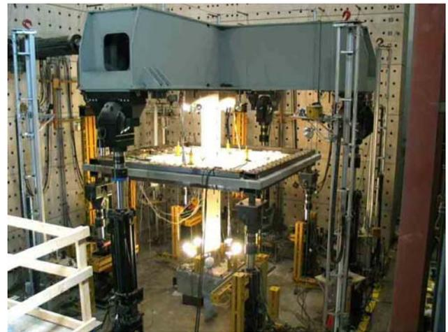
Slab-column subassembly at NEES MAST facility. Photo courtesy of the MAST laboratory.
