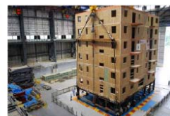
The capstone test structure is moved onto the E-Defense shake table in Japan on June 22, 2009. Photo courtesy of John van de Lindt, Colorado State University.
