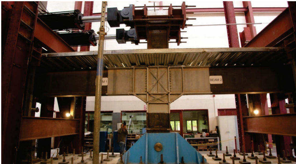
Figure 5-3 Sample interior frame test specimen with composite slab (NIST, 2016).
