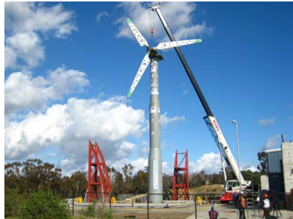
Figure 7. Testing the response of a wind turbine to seismic shaking at UC San Diego NEES facility. © 2010. UC San Diego. Used with permission.
