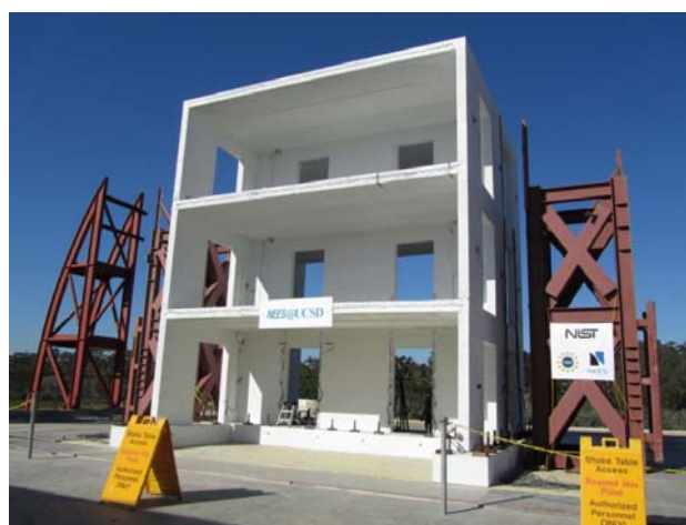
Figure 5. Full-scale seismic testing of a three-story building design in the NEES facility at UC San Diego. © 2010. University of California, San Diego. Used with permission.
